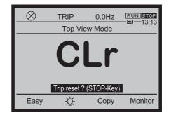
When you press the [STOP/RESET] key again while "CLr" is blinking, the trip is reset. The display on the screen once disappears, and the screen immediately after power on is displayed.
